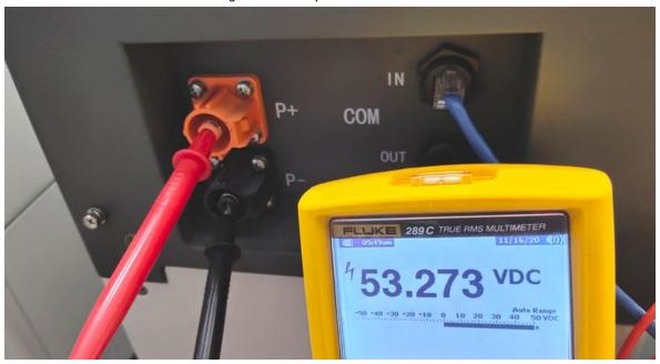
The voltage measured on the PDU is the combination / average voltage of all modules in the tower. This should be around 50 V. If it is not around this value, please measure the voltage of each individual LVS Module by one of the following two possibilities (please note, that you cannot measure the correct voltage in any other way).
